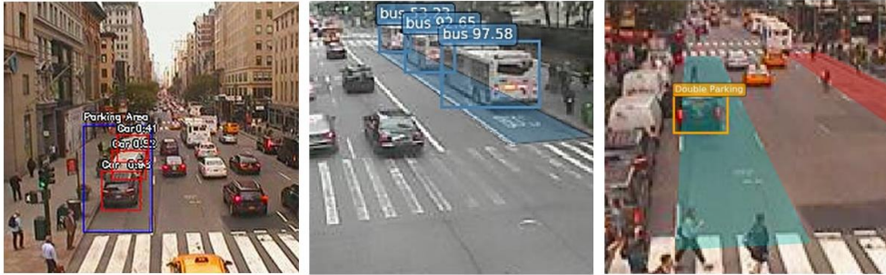
(a) Detect Parking Occupancy (b) Monitor Bus Lane Usage (c) Identify Double Parking
